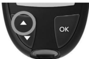
2. Press and HOLD the **▲** button for about 3 seconds, until you see the blinking **Bluetooth** symbol (as shown in the next step). A blue light blinks when you are in pairing mode.
