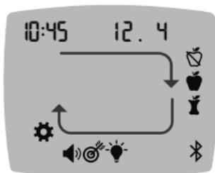
4. To scroll through **Settings** options as shown in the image, press the ▲ or ▼ button until the symbol you want is blinking.
