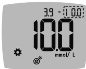
5. To change the blinking **High** end of the **Overall Target Range**, press the **▲** or **▼** button.
