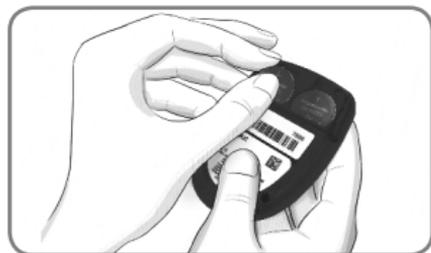
4. Make sure the '+' sign is facing up on the new batteries.
