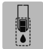
The meter turns on, displaying a test strip with a flashing blood drop.
