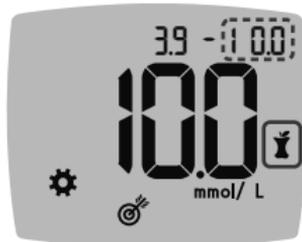
7. To change the blinking **High** end of the **After Meal Target Range**, press the ▲ or ▼ button.
