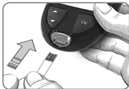
2. Insert the grey square end firmly into the test strip port until the meter beeps.
