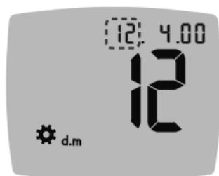
6. To change the day (blinking), press the ▲ or ▼ button, then press **OK**.
