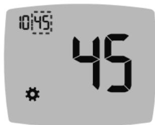
5. To change minutes (blinking), press the ▲ or ▼ button, then press **OK**.
