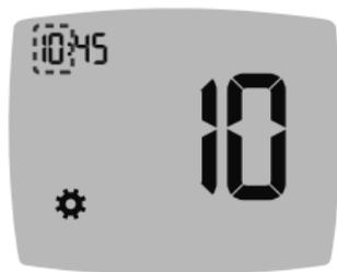
4. To change the hour (blinking), press the ▲ or ▼ button, then press **OK**.
