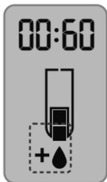
1. If the meter beeps twice and the screen displays a blinking blood drop with a plus sign, the test strip does not have enough blood.
