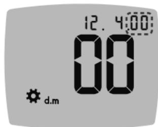
4. To change the year (blinking), press the ▲ or ▼ button, then press **OK**.
