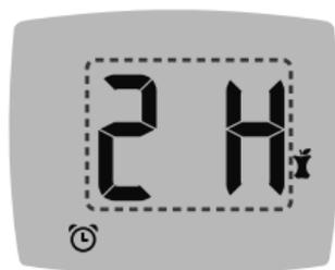
3. To scroll from 2 hours to 0.5 hours by half-hour intervals, press the ▲ or ▼ button.
