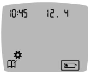
When the batteries are low, the meter operates normally, displaying the **Low Batteries** symbol until you replace the batteries.
