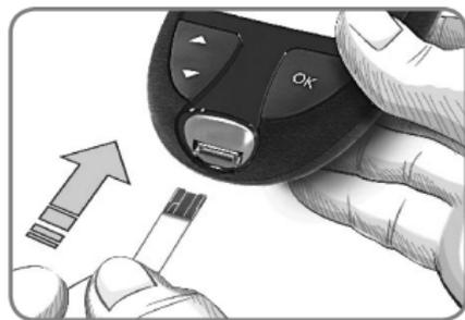
2. Insert the grey square end of the test strip into the test strip port until the meter beeps.
