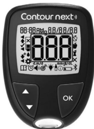
All symbols on the screen and the white strip port briefly light up. Verify that the meter screen fully displays **8.8.8** and that the white light from the test strip port is visible.
