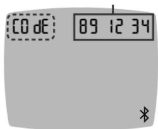
When a connection is made, the meter displays the 6-digit pass code.
