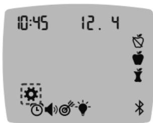
6. To exit from the **Settings** menu and return to the **Home** screen, press the ▲ or ▼ button until the **Settings** ⚙️ symbol is blinking.
