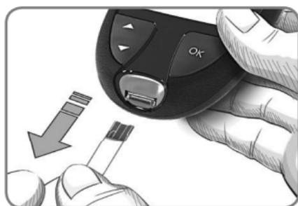
To turn the meter off, remove the test strip.
