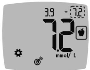
5. To change the blinking **High** end of the **Before Meal Target Range**, press the **▲** or **▼** button.
