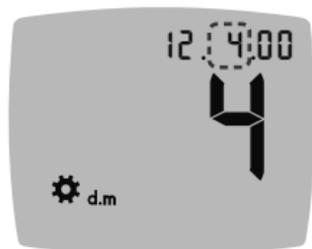
5. To change the month (blinking), press the ▲ or ▼ button, then press **OK**.
