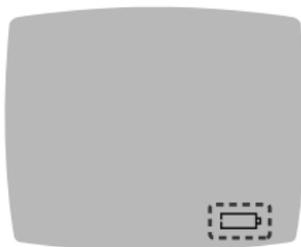
When you are no longer able to perform a test, the meter displays the **Dead Batteries** screen. Replace the batteries immediately.
