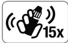
3. Shake the control solution bottle well, about 15 times before every use. Unmixed control solution may cause inaccurate results.
