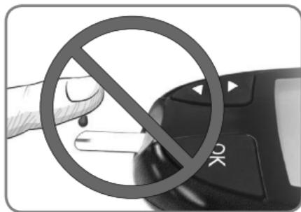
**CAUTION:** Do not press the tip of the test strip against the skin or place the blood on top of the test strip. This could lead to inaccurate results or errors.
