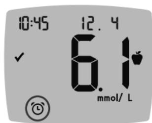
The screen returns to the **Before Meal** reading. The meter displays the **Reminder** (🕒) symbol to confirm the Reminder is set.
